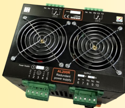
AL200R redundant two 230Vac inputs one 127Vdc output 2x 1000W
